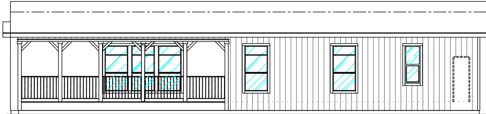
Rear Sidewall Elevation (SHOWN WITH TALL WINDOWS)
